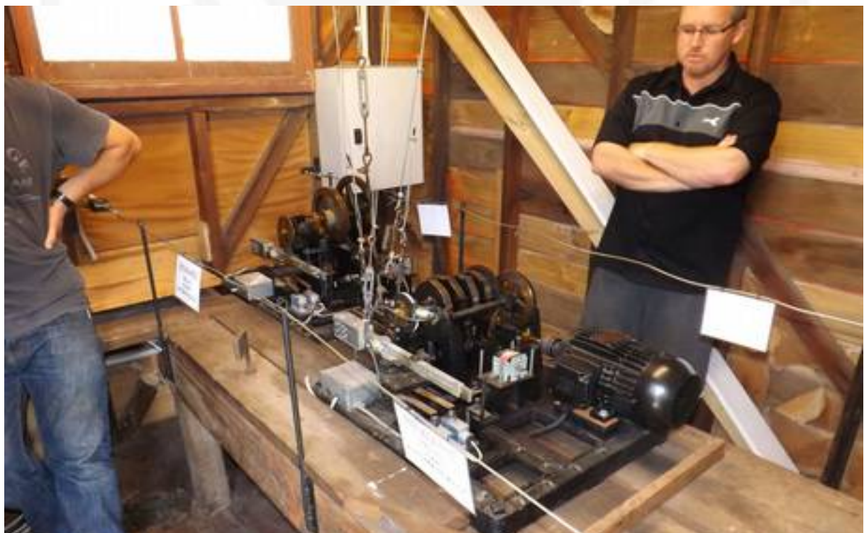
Cooks Gardens Bell Tower Chime Mechanism
